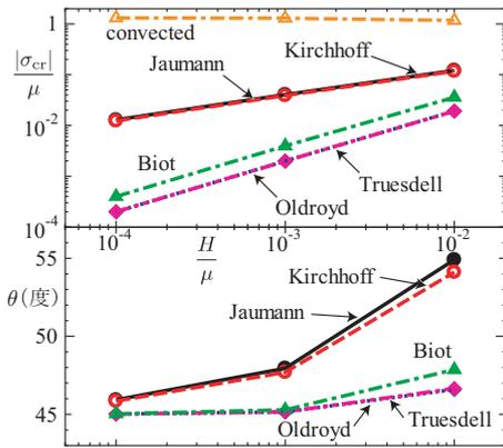
図-1 圧縮時の  $H/\mu$  の影響 ( $\alpha = \beta = 0, \bar{\mu}/\mu = 0.1$ )
