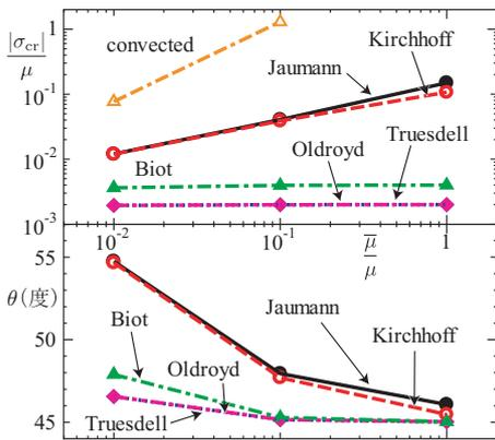
図-2 圧縮時の  $\bar{\mu}/\mu$  の影響 ( $\alpha = \beta = 0, H/\mu = 0.001$ )
